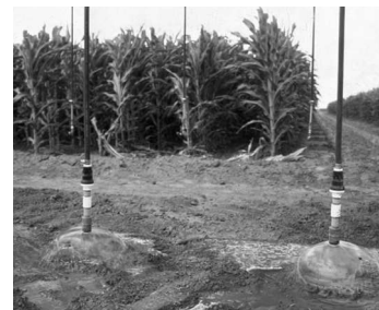
Figure 6. LEPA center pivot with a bubble applicator on corn.
