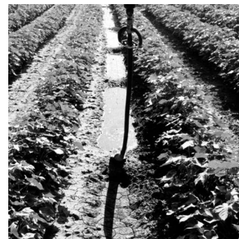
Figure 5. LEPA center pivot with a drag sock.
